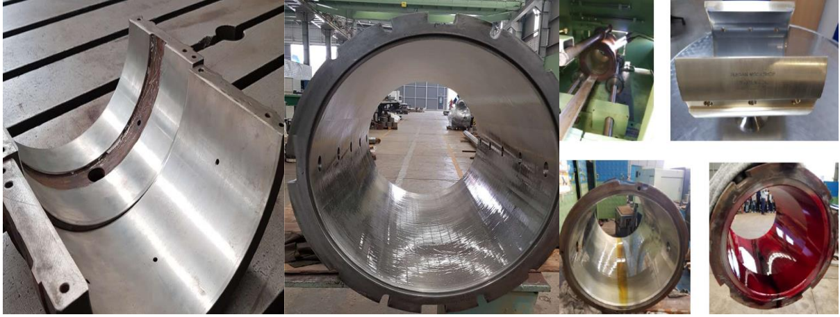
Figure 46 - Class Approved Re-metalting (White Metal) Application - Tersan Shipyard
