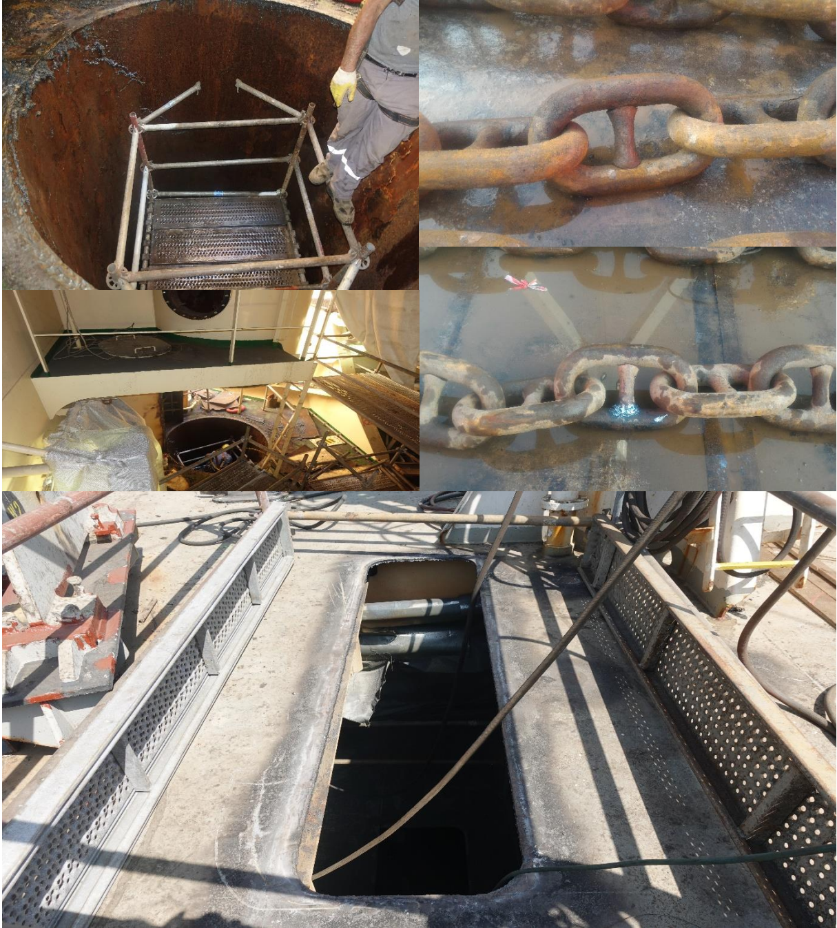
Figure 63 - Chain & Chain Locker Steel Renewal Process
