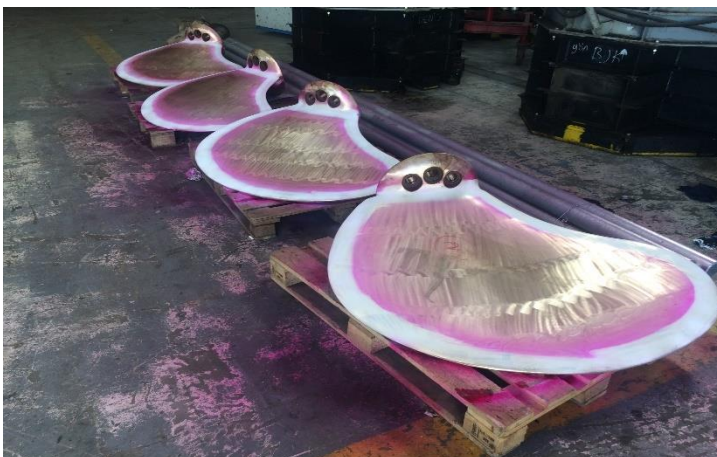
Figure 50 - Propeller Blade Root & Edge Crack Test – Desan Shipyard
