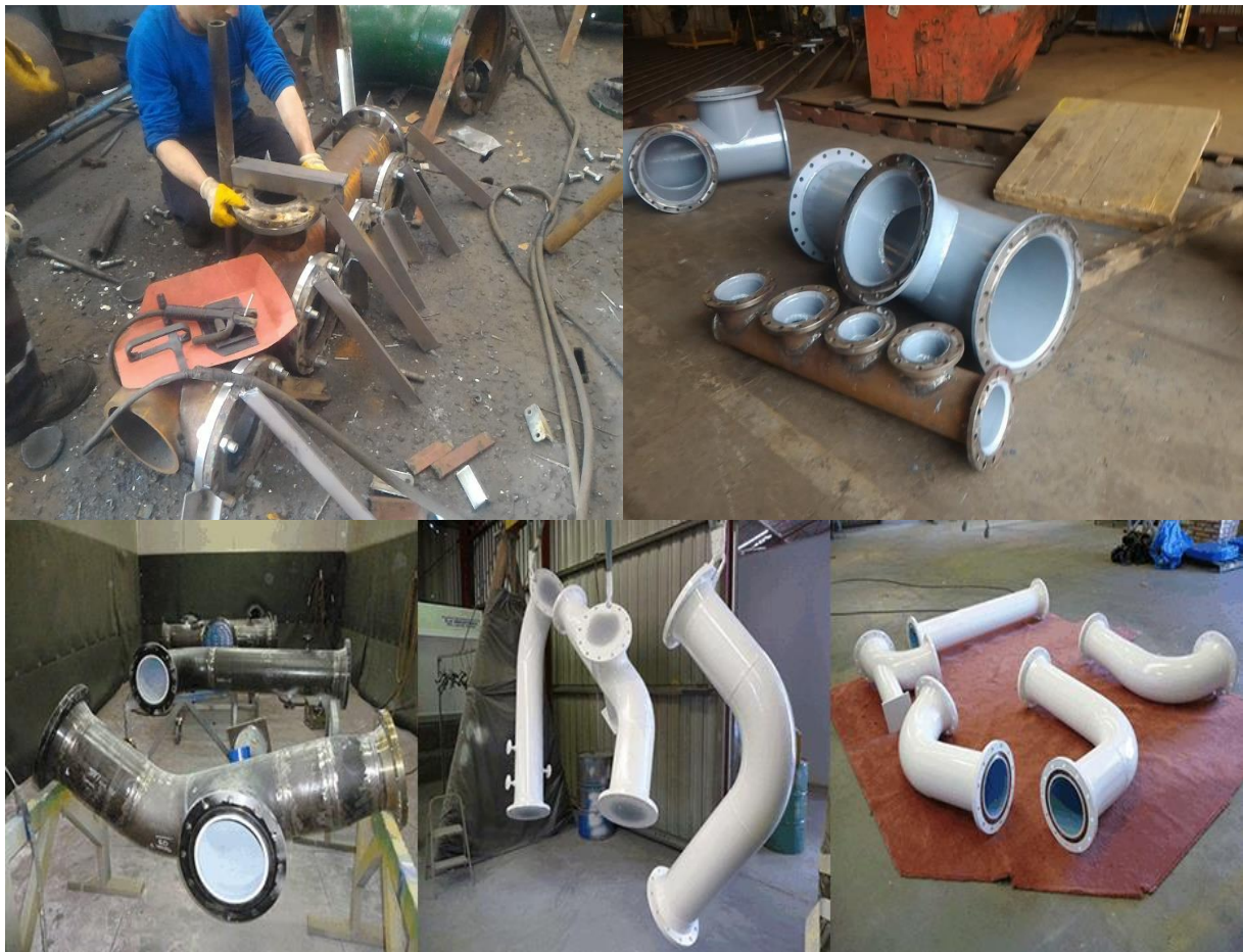
Figure 119 - Pipe Fabrication in Workshop with Coating (RS 500P + RA 500M – Glassflake Epoxy)
