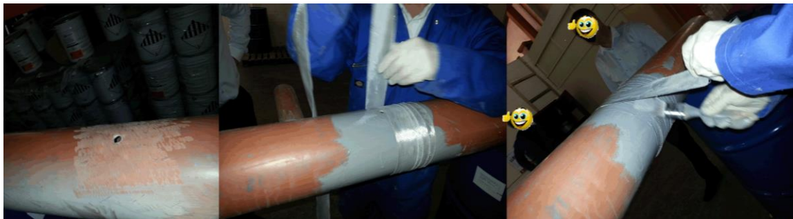
Figure 132 - Application of Cold Repair System on GRP – GRE Pipe Samples
