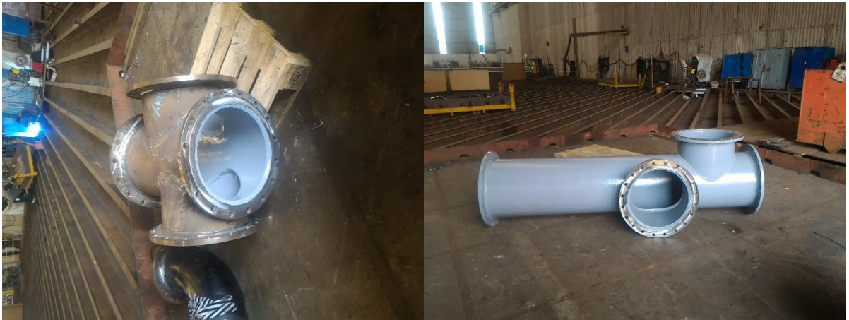
Figure 222 - Prefabricated Pipe Inner Coating (RS 500P + RA 500M Glassflake Epoxy)
