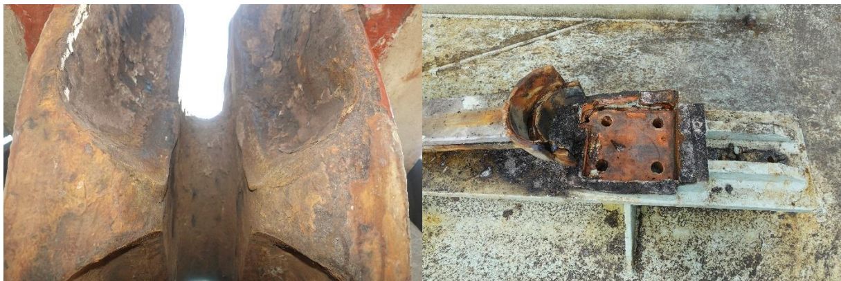
Figure 69 - Windlass Repairs – Chocking Compound Application
