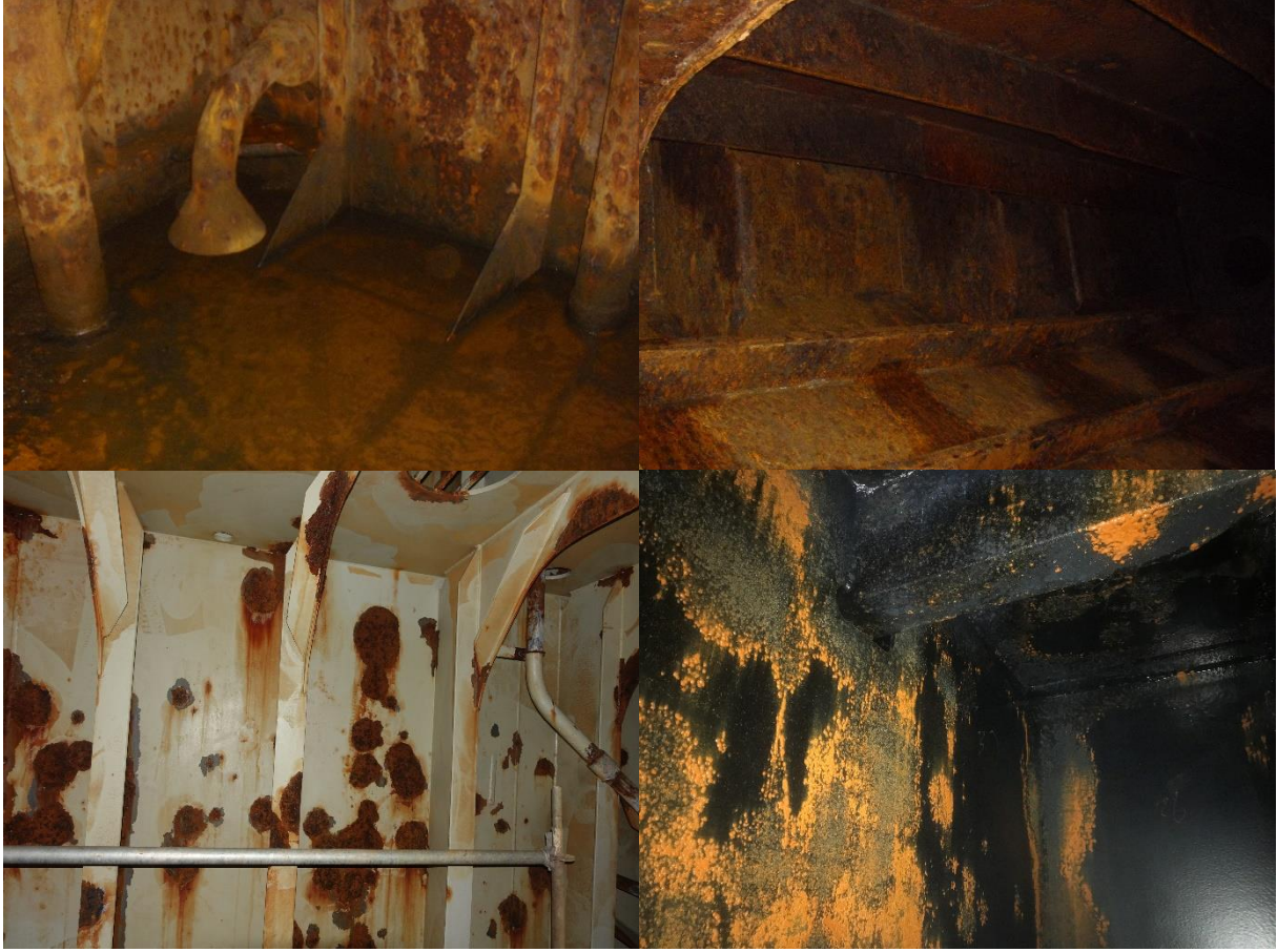
Figure 80 - Ballast Tank Condition (Poor)
