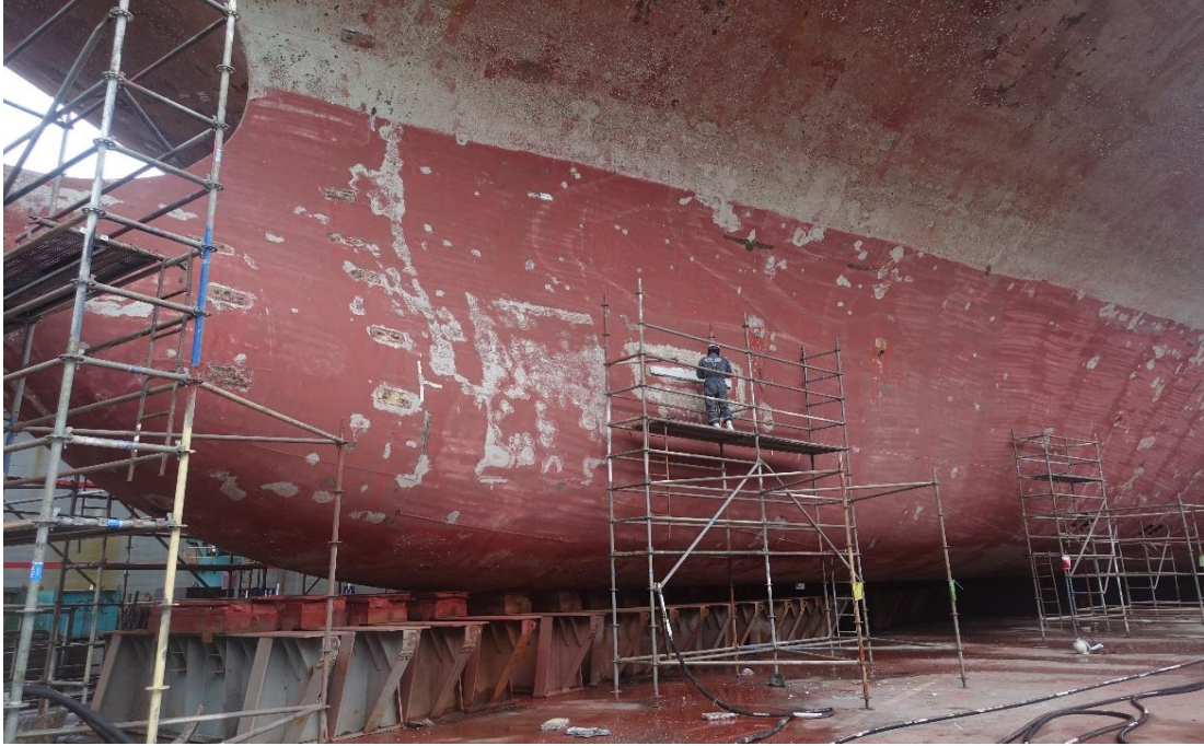
Figure 56 - ICCP Anode Filler Application (RS 500P + RA 500M with Spray – Dielectric Shield)
