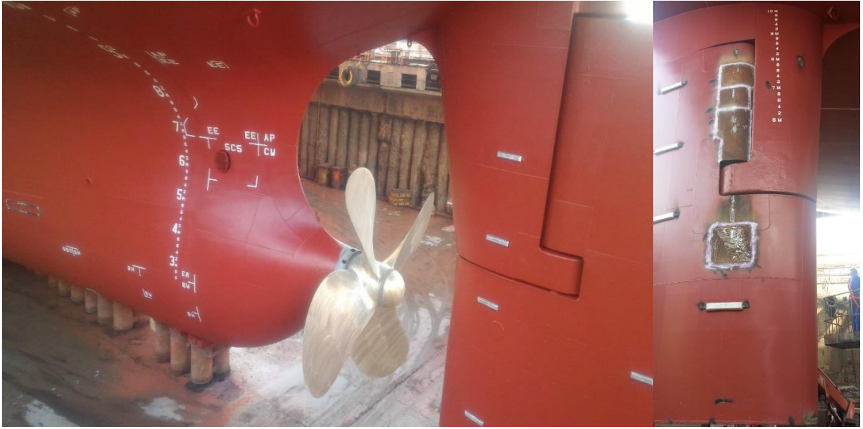
Figure 54 - Stern View & NDT Application on Rudder Welds
