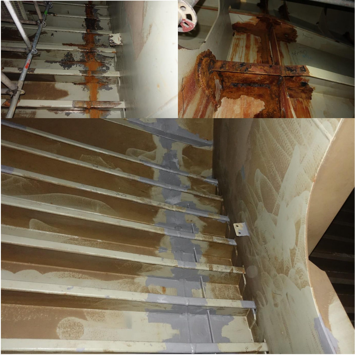
Figure 182 - Waterjetting of Block Erection Points and RS 500P Application
