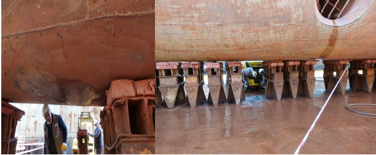
Figure 58 - Speed Log & Echosounder Position Check – Keel Block Removal
