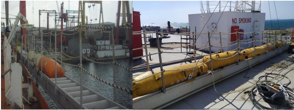
Figure 208 - Load Testing of Ladders with Weight Bags
