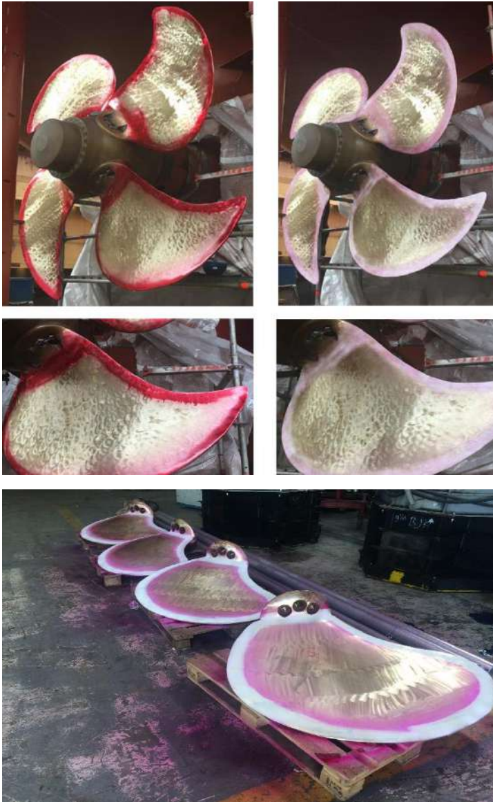
Figure 49 - Propeller Blade Root & Edge Crack Test – Desan Shipyard
