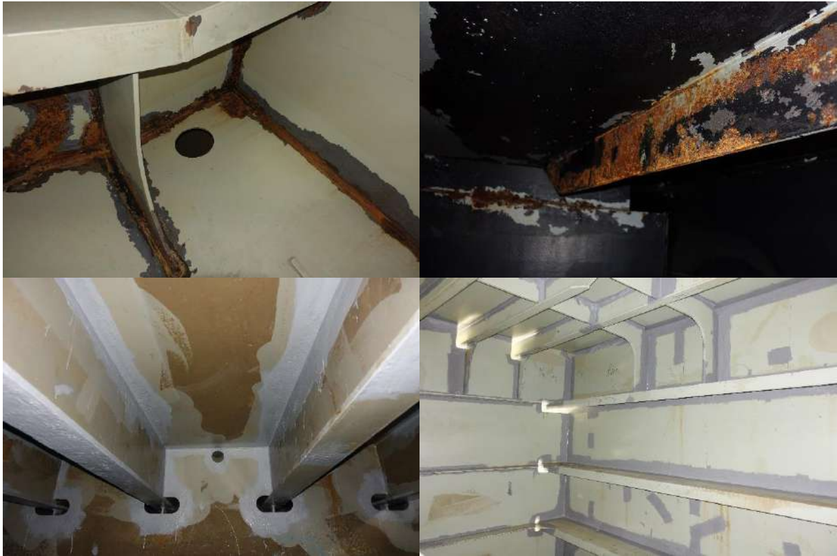
Figure 180 - Waterjetting & Spot Coating Application for Ballast Tanks
