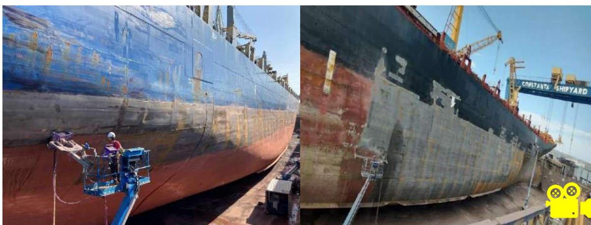
Figure 157 - Waterblasting by Falch (3000 bars 45 liter) WJ1 - WJ2 (~SA2 - SA2½)
