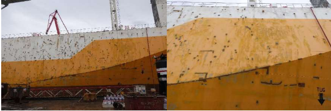
Figure 154 - Hull Blasting Damages with Spot Blasting
