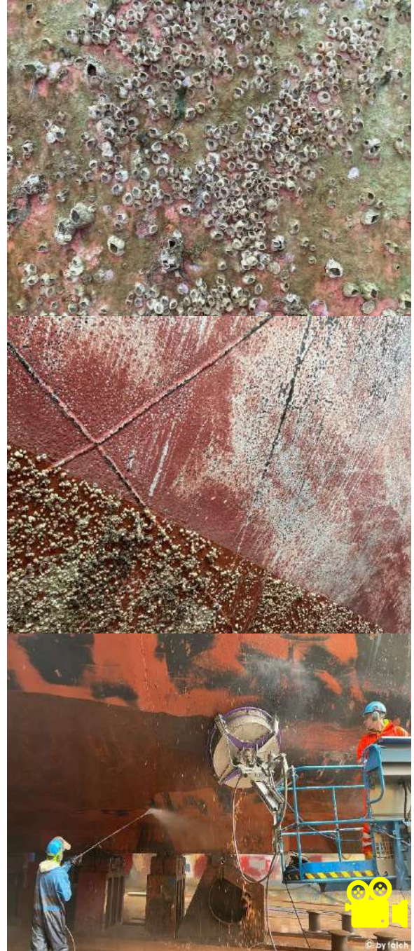
Figure 161 - Helijetting for Hull Washing @500 bars
