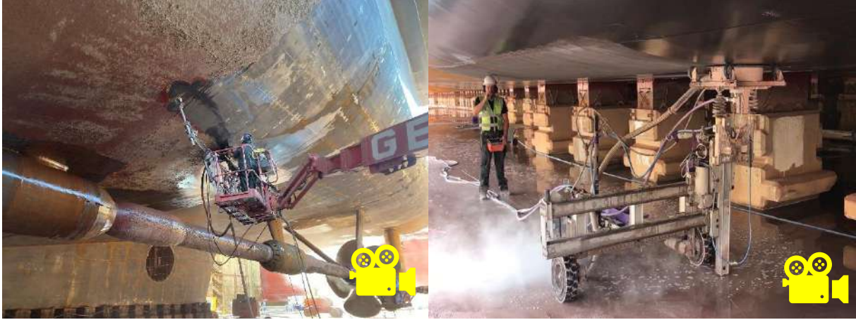
Figure 164 - Hull Waterblasting with Falch Robots (3000 bars 45 liters)
