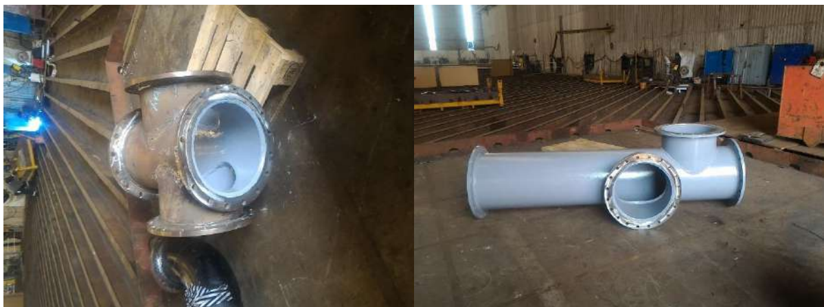
Figure 223 - Prefabricated Pipe Inner Coating (RS 500P + RA 500M Glassflake Epoxy)
