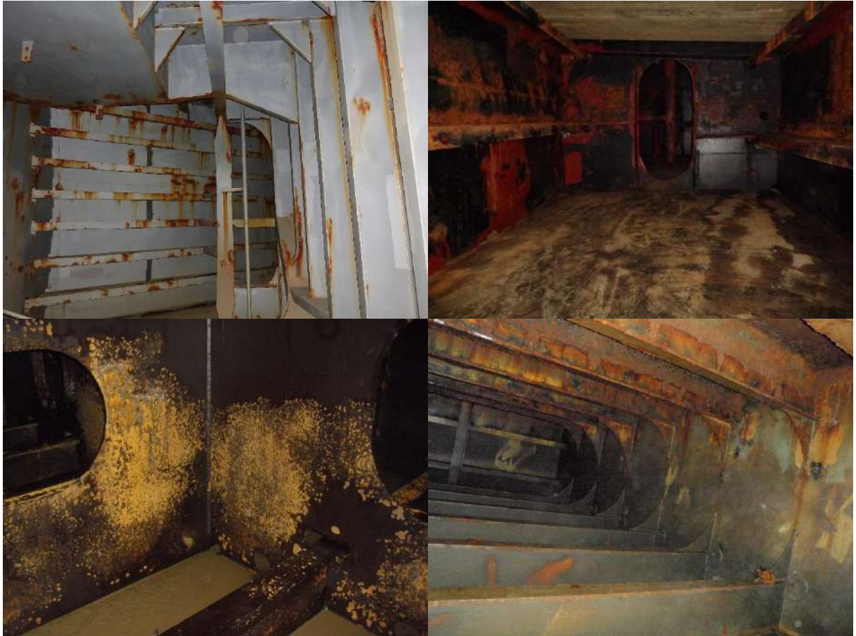
Figure 176 - Ballast Tank Condition (Rust & Blisters)
