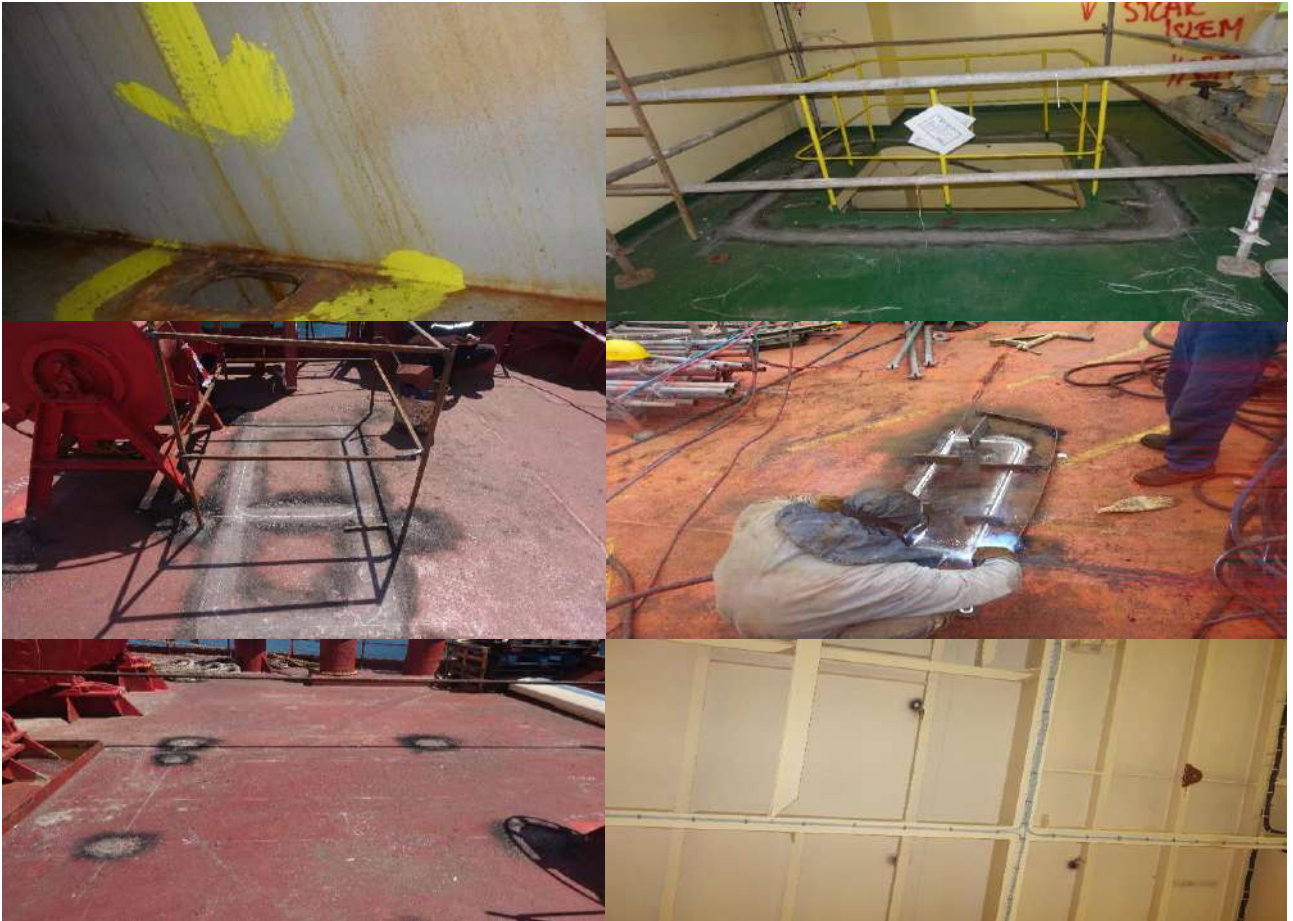
Figure 87 - Marking of Steel Plates Before Cropping
