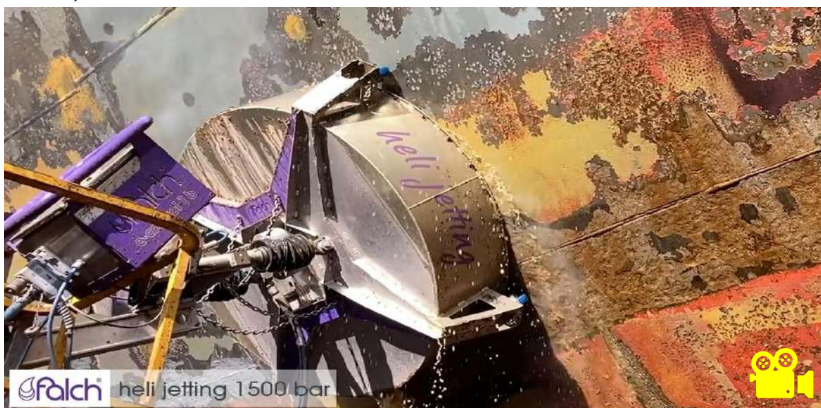
Figure 158 - Helijetting System by Falch (1500 bars) Spot Blasting (WJ3 - WJ4 ~ SA1 + Sweeping)
