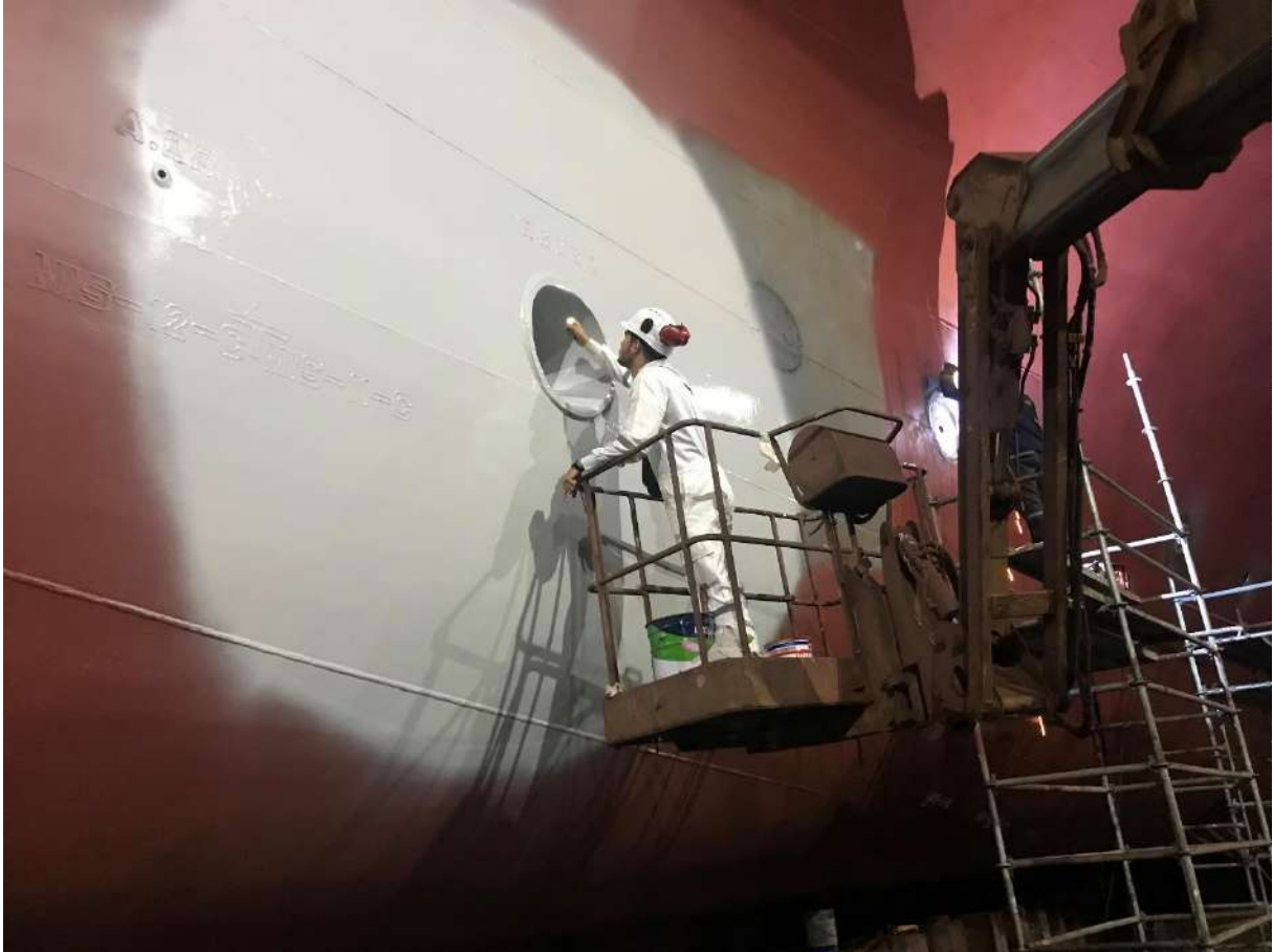
Figure 42 - Overboard Pipe Inspection ( Scrubber Overboard with Glassflake RA 500M )
