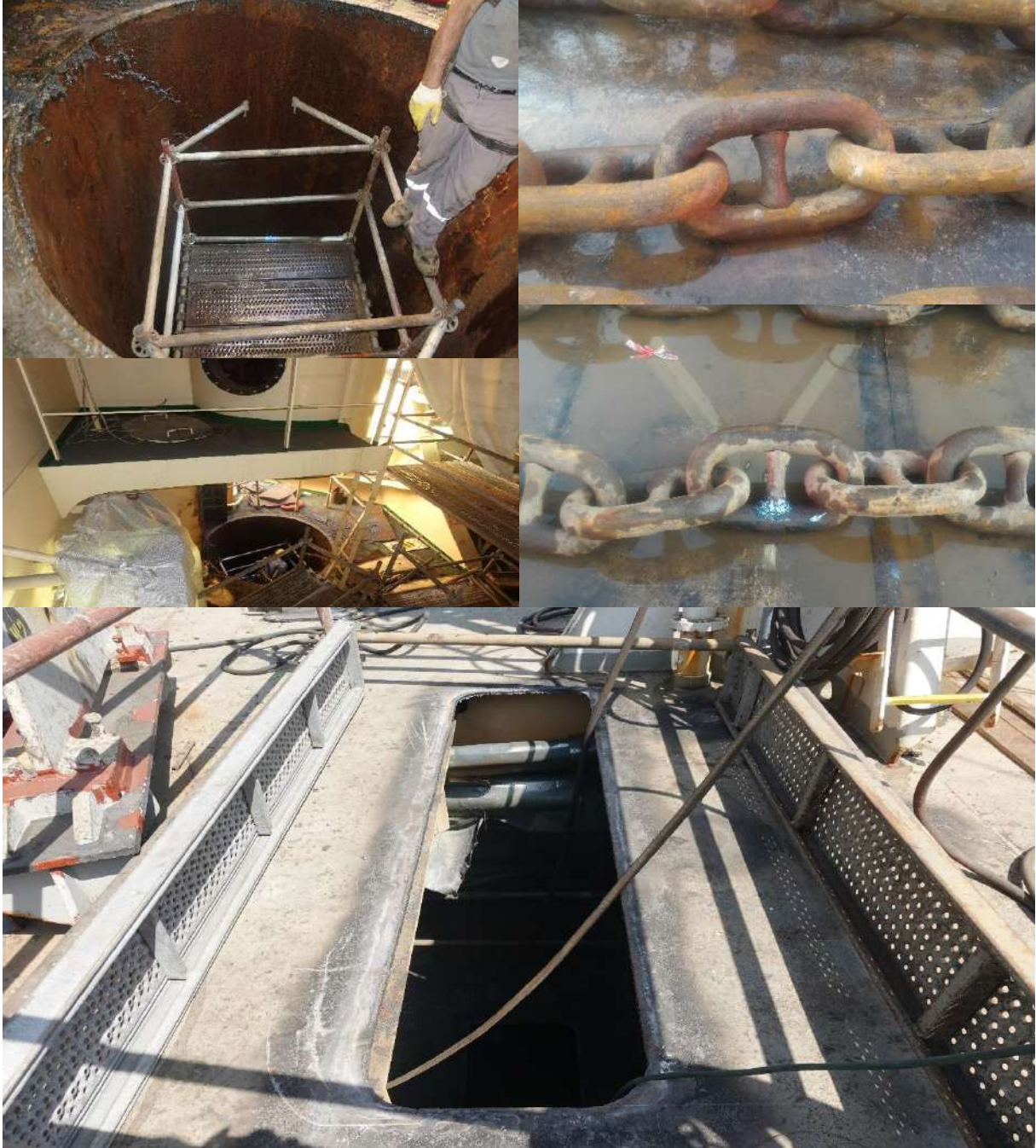
Figure 63 - Chain & Chain Locker Steel Renewal Process
