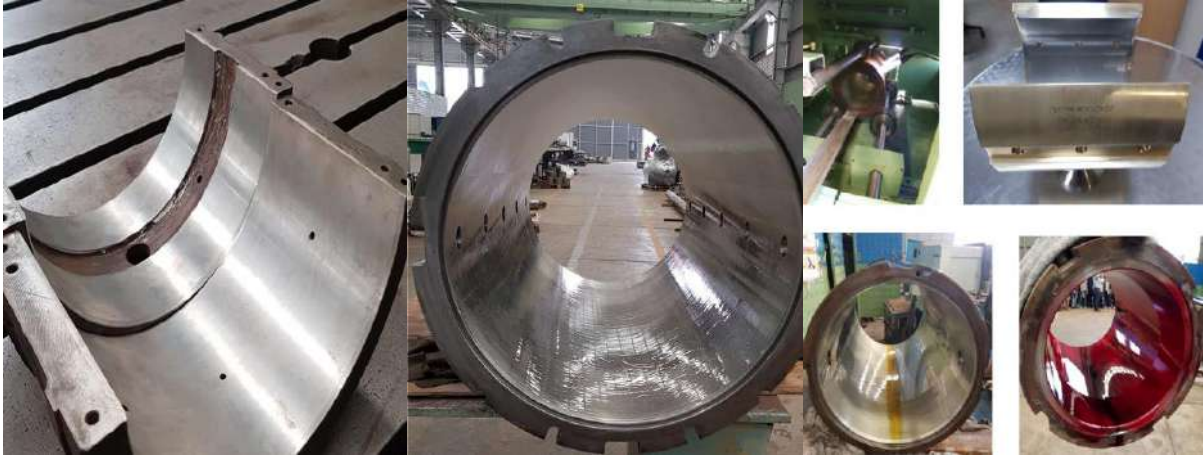
Figure 46 - Class Approved Re-metaling (White Metal) Application - Tersan Shipyard
