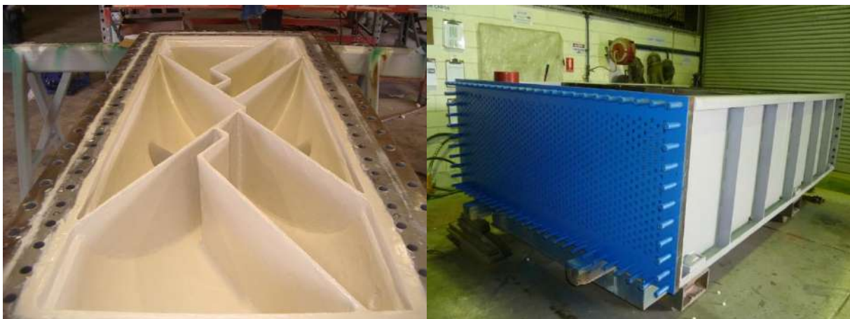
Figure 66 - Cooler Case Glassflake Application (Chemco RS 500P + RA 500M Glassflake Epoxy)
