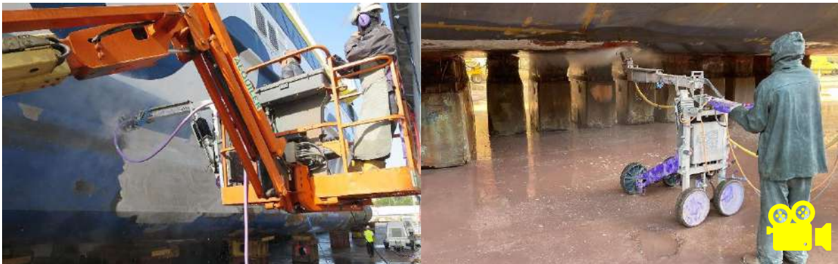
Figure 165 - Hull Spot Repairs With Multiworker
