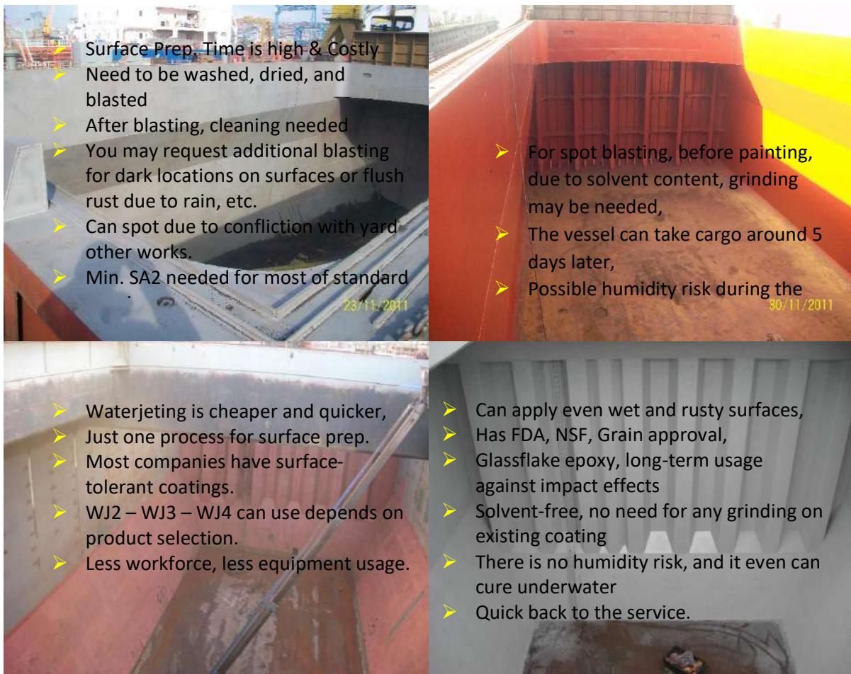
Figure 175 - Hold Coating Application
