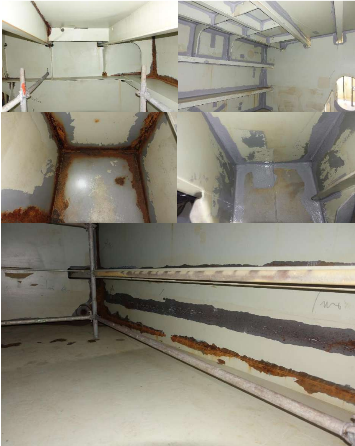
Figure 181 – Waterjetting (500 – 800 bars) of Ballast Tanks and RS 500P Application on Wet & Rusty Surfaces
