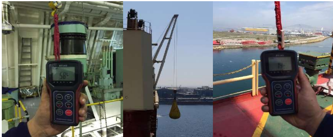
Figure 203 - Load Test of Cranes
