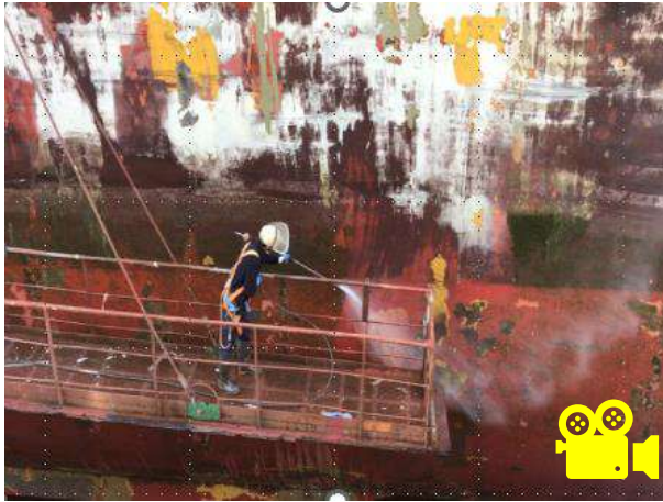
Figure 162 - Manuel Hull Washing (Unsafe – Low Efficiency and Low Quality)
