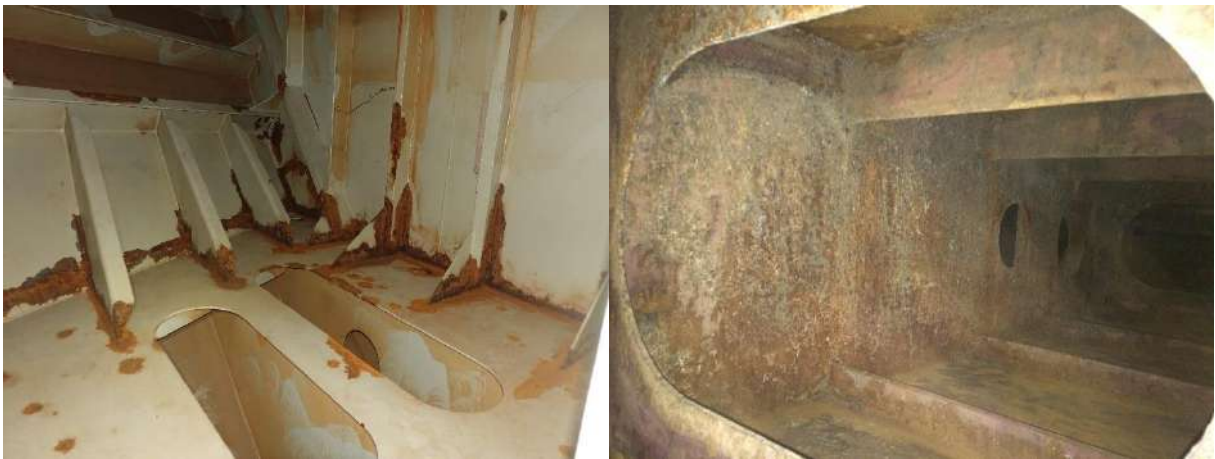
Figure 178 - Waterjetted Ballast Tanks
