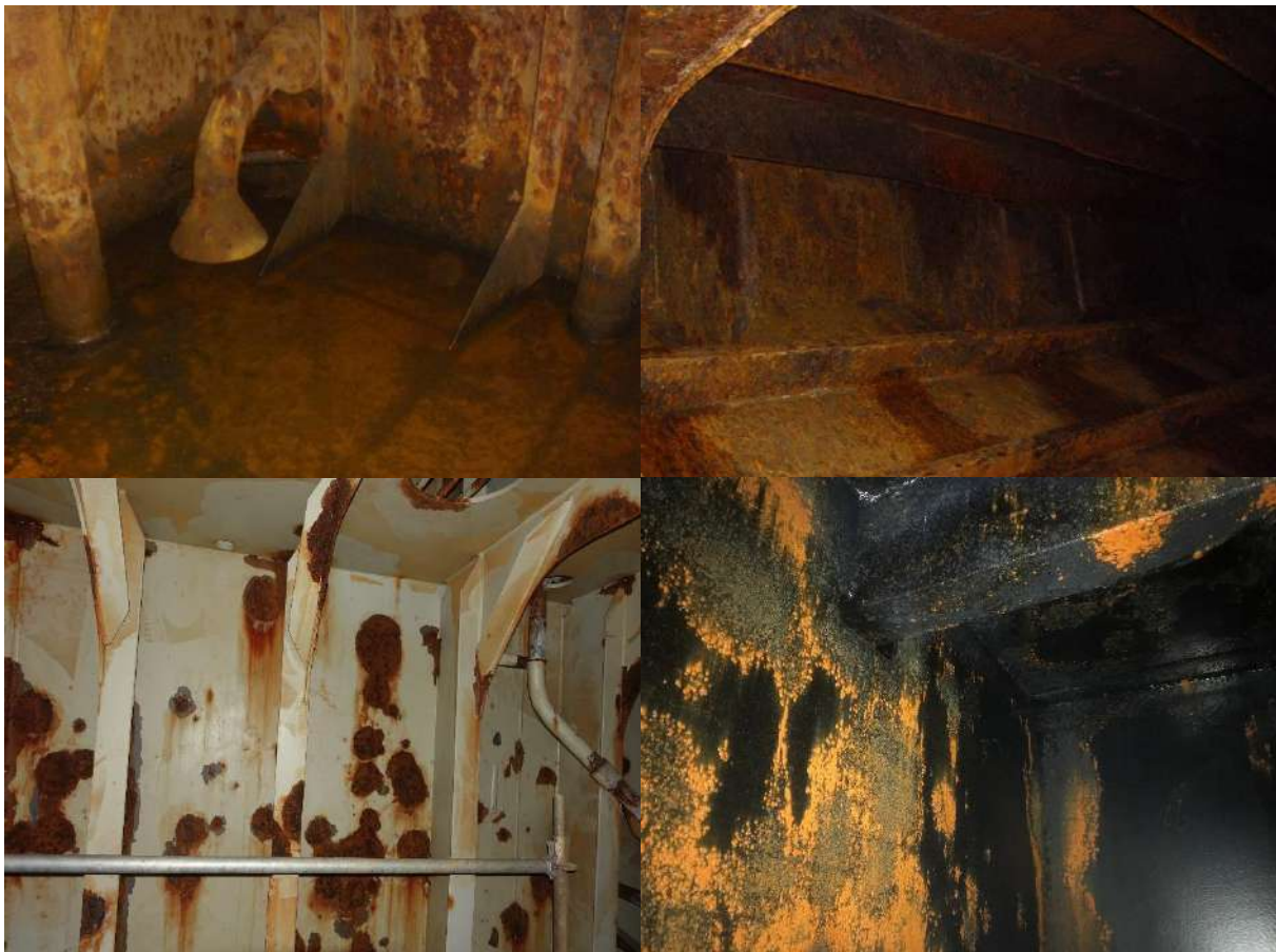
Figure 80 - Ballast Tank Condition (Poor)
